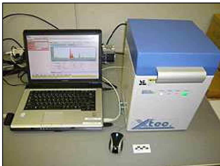
On-site Soil Contamination Analyzer
